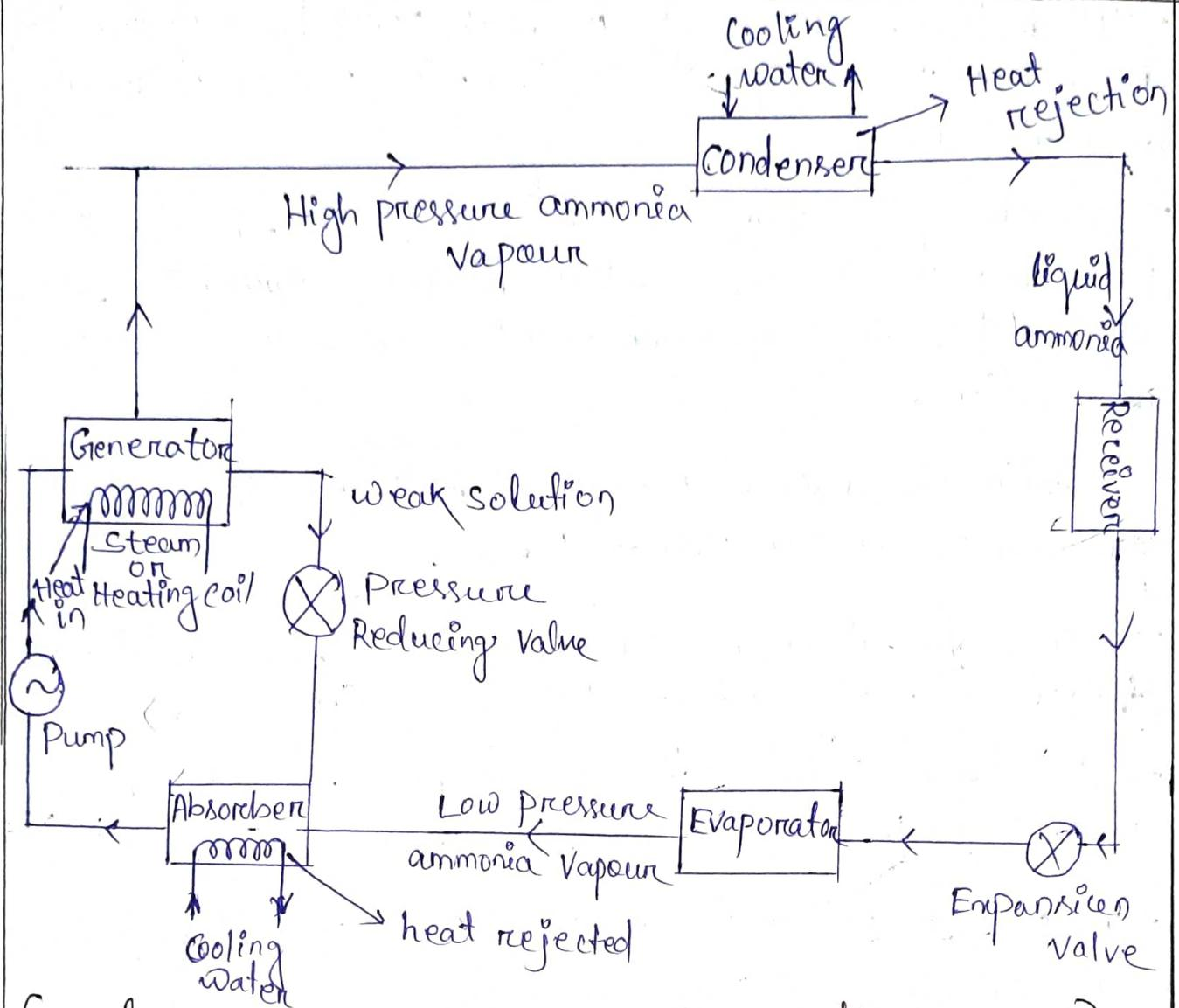
(Simple vapour absorption refrigeration system)
