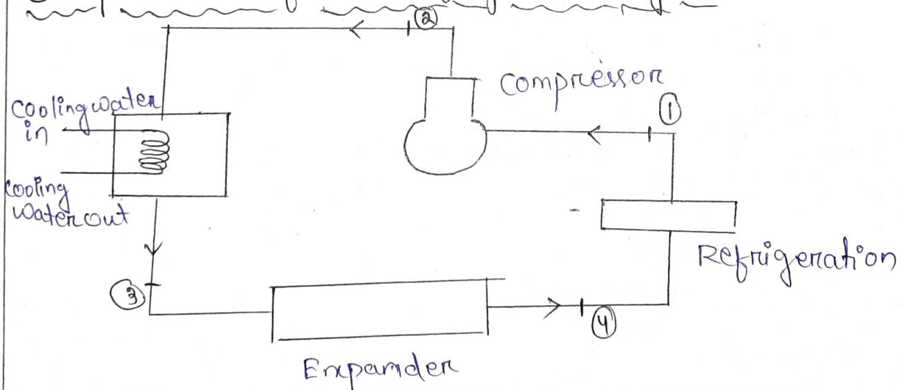
The main components of air refrigeration cycle are.
