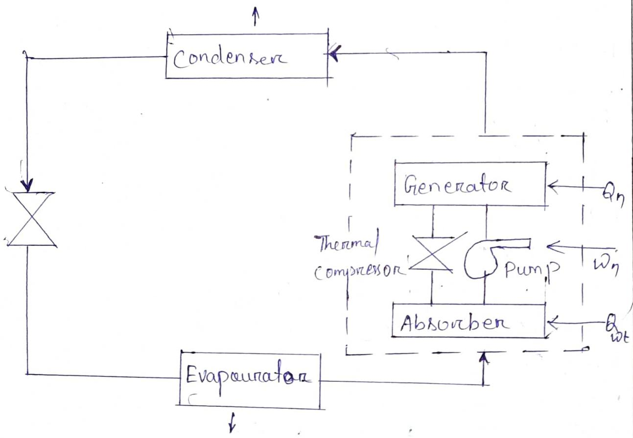
(Simple vapour absorption Refrigerator system)
